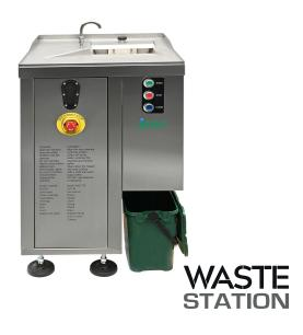
Food waste typically represents around 40% of total commercial catering waste. Of this 40%, approximately 77% is liquid. The WasteStation Compact grinds the food waste into fine particles, these particles feed directly into the built-in dewatering system. Through centrifugal action, the WasteStation forces out the excess liquid from the macerated waste.
