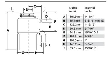
**NOTE:** Plumb 38.1 mm (1-1/2") waste line to prevent standing water in disposer motor housing.
