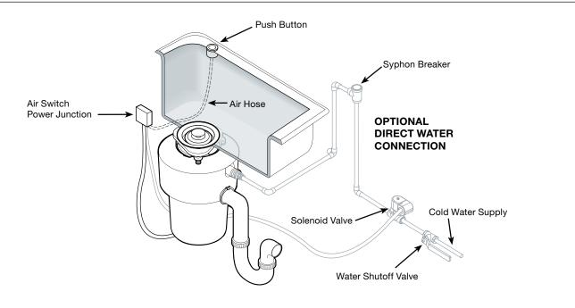
**PLEASE NOTE:** The Air Switch and socket need to be purchased seperately. For the wall mounting option a 20A ground connection is needed.
