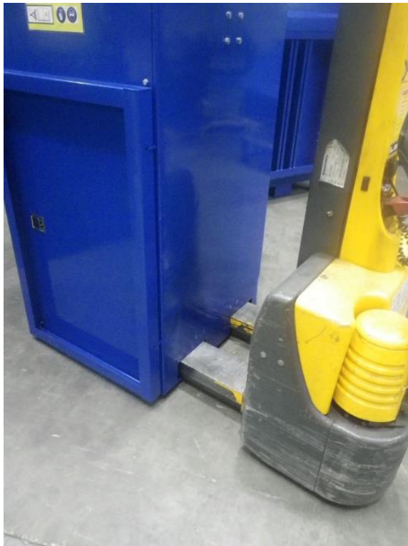
Fig. 1: The prongs of the forklift are inserted into the lifting channels for a safe and secure handling of the machine. Do not tilt the machine more than 8°
